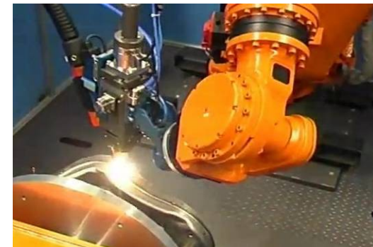
Hybrid Laser Welding Images Courtesy of SMU: Center for Laser Aided Manufacturing
